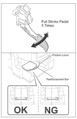
e) Pump the accelerator pedal 5 times in a full stroke to properly seat the reinforcement bar.
